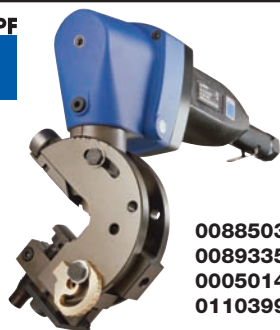
1439361 Punch 1439360 Carrier with Integrated Die
